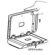
1 Open TFT cover first, then press OPEN button to open the disc cover.
